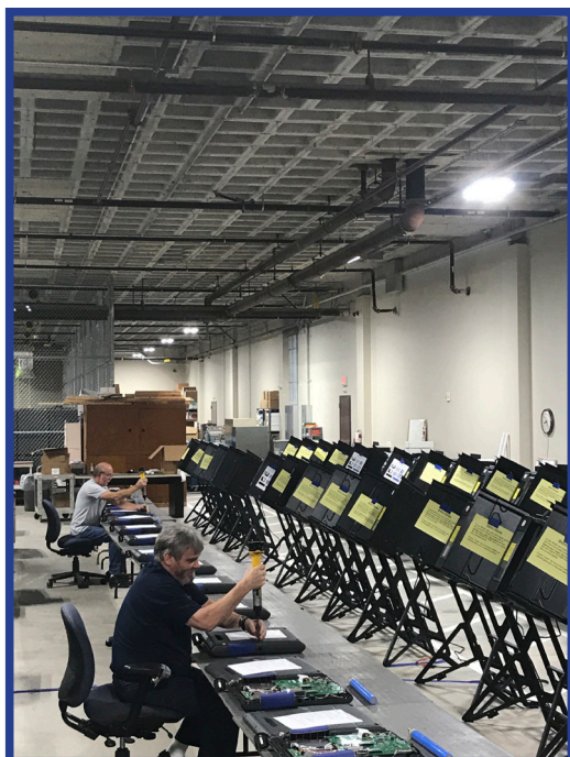
Warehouse Supervisors, Joe Winter and Craig Hite, repair iVotronic Voting Machines
